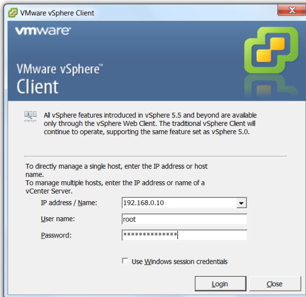
Figure 8: Connecting to the server using the vSphere client
